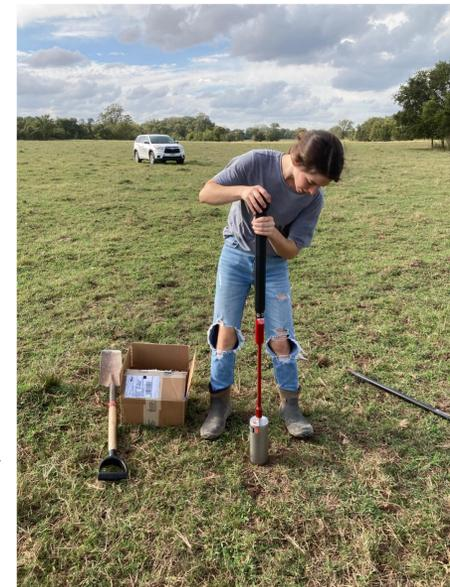
Figure 3. Sample collection using slide hammer
