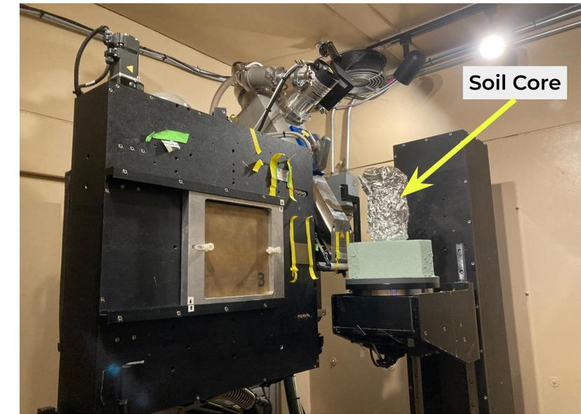
Figure 4. Soil core inside the North Star Institute (NSI) Scanner System at University of Texas CT Lab
