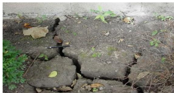
Figure 2. "Cracks in expansive soils"
