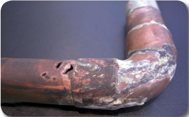
**Figure 2.** Pinhole leaks in copper tubing caused by internal corrosion.
