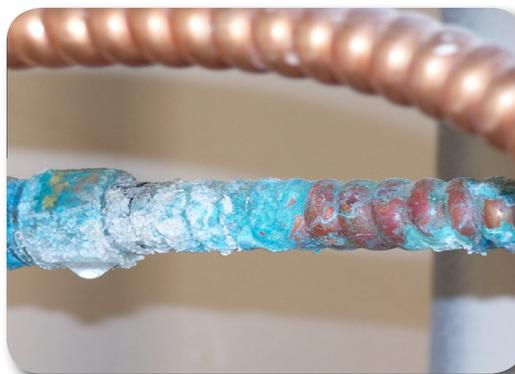
**Figure 1.** Corrosion at a connection on a water heater indicated by the blue-green color.
