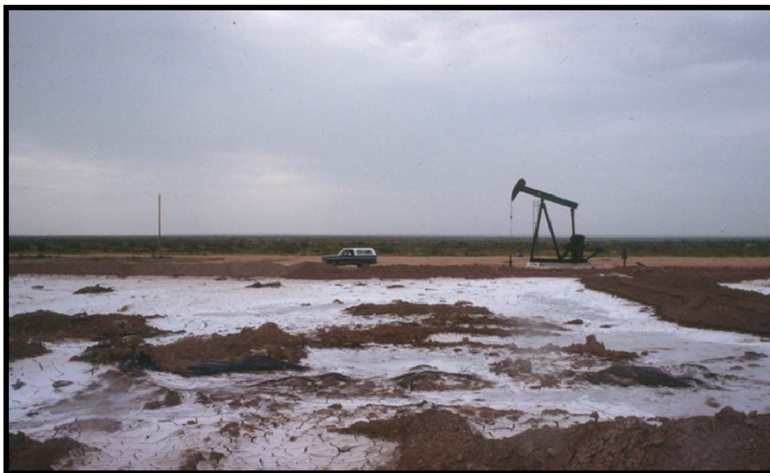
Photo 3. Salt accumulation on the surface of the soil at a reserve pit.
